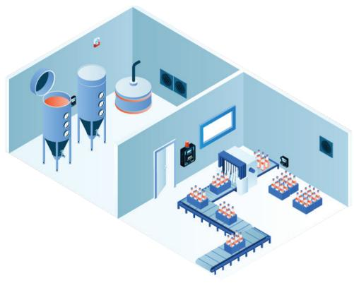
During the bottling process, CO<sub>2</sub> is used to pre-fill each bottle before it is filled with beer. Another CGAS Detector with a CO<sub>2</sub> infrared sensor should be mounted in the bottling area to monitor and protect workers on the bottling line. The cGas Detector CO<sub>2</sub> transmitter is available with analog output (p/n:
