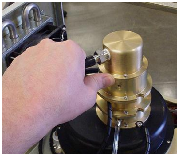
Figure 6-2 Disconnect Sample Inlet Tube
