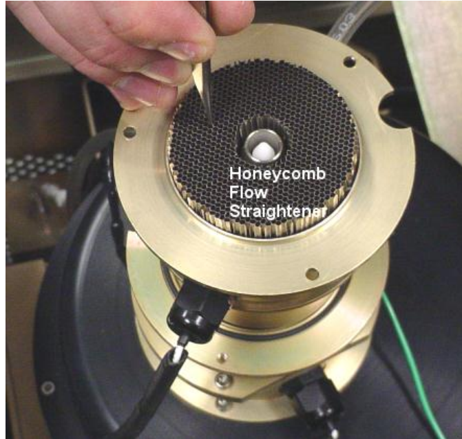
Figure 6-5 Remove the Honeycomb for Reassembly
