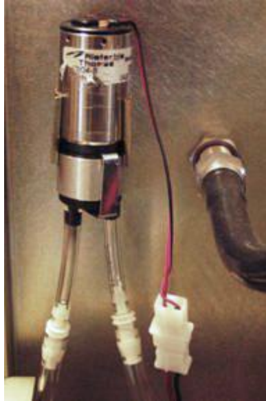
Figure 6-24 Extraction Pump Location (inside back panel)
