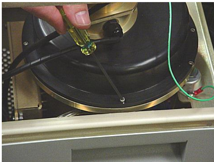
Figure 6-10 Unscrew Charger Head Assembly Screws
