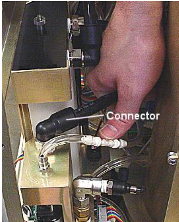
Figure 6-17 Disconnect the Sheath Air Hose
