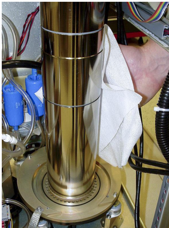
Figure 6-21 Clean the Center Column
