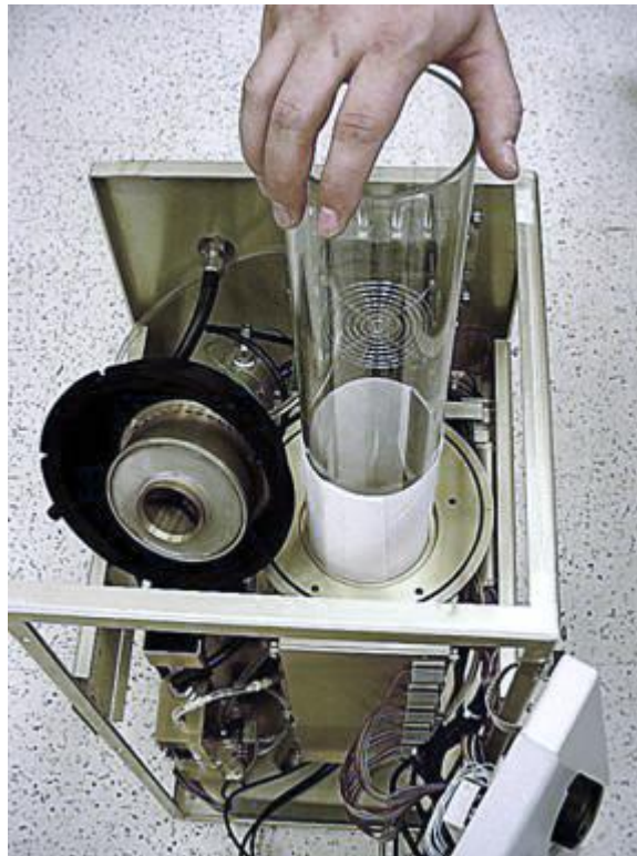
Figure 6-13 Cleaning the Charger Column
