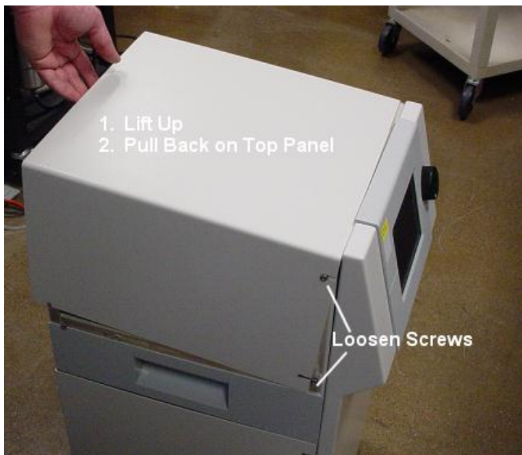
Figure 6-1 Remove Top Panel
