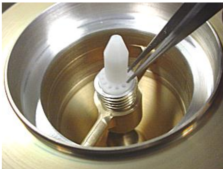
Figure 6-7 Hold the Flange with Tweezers
