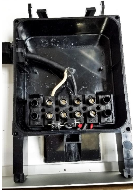
Figure 11: Secure Terminal Block and Tighten Strain Relief
