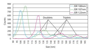
Typical resolution is within 2.5% of the particle diameter at 0.1  $\mu m$  . The Model 3340A can differentiate between 100 nm and 107 nm PSL!
