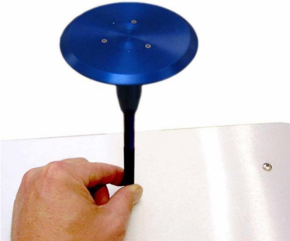
Figure 6: Thread the Inlet into the Inlet Ring after Heat Shield is Installed
