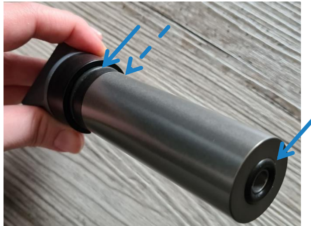
Figure 4: Sealing Rings at the Alcohol Cartridge
