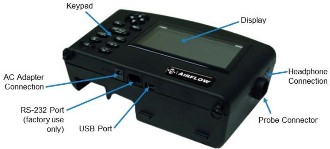
Figure 1: Features of the PH730/PH731 Micromanometer, Front View
