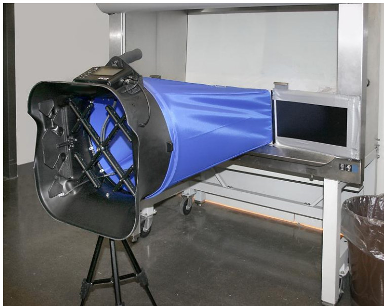
Figure 23: Direct Inflow Measurement Hood
