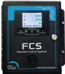
The FCS-8 is a sophisticated, high performance system controller that offers up to 8 gas channel configurations for monitoring toxic, combustible or refrigerant gases with versatile control functionality for non-hazardous, non-explosion rated, commercial and light industrial applications. The FCS-8 is designed to accept inputs from digital and/or analog transmitters and/or Peripheral Devices (in various combinations), using Modbus® RTU RS-485 or 4-20 mA analog input.
