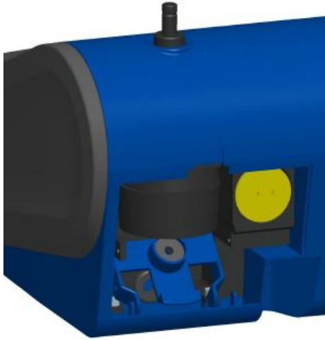
Figure 4-7: Open Blue Retention Clip
