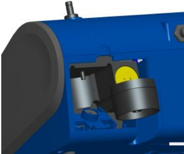
Figure 4-8: Remove 37-mm Filter Cassette
