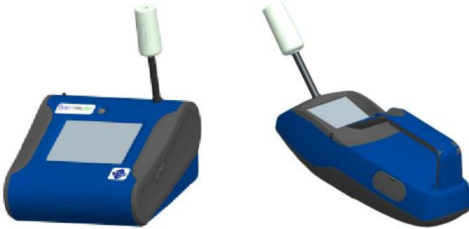
Figure 4-1: Attach Zero Filter to Inlet
