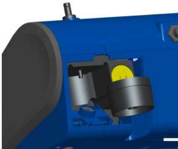
Figure 4-8: Remove 37-mm Filter Cassette
