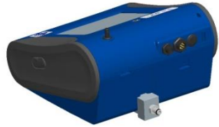
Figure 2-4: Connect Exhaust Adapter to Exhaust of DustTrak™ Monitor
