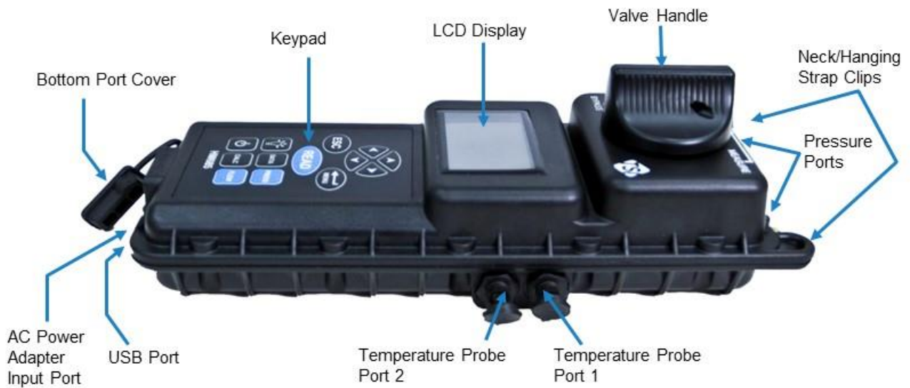
Figure 1-1 HM685 Meter Description
