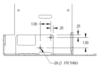
5. Then use two 6-32 locking nuts on the back side of the flange when attaching the "Mounting Bracket."
