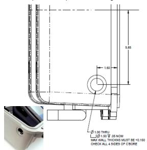
The Environmental Enclosure Bracket may need two holes added. Check the back left section of the large black sheet metal bracket for the installed 6-32 PEM nuts.
