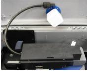
Attach Temp/RH Grommet to Case.
