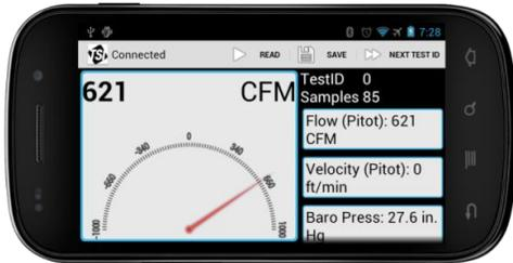
Utilizing wireless Bluetooth® technology, this app for Android™-based smartphones and tablets communicates with the instrument remotely over 100 ft. (30.5 m) away and displays sample data in real time. Attach comments, voice notes, and photos to test ID data for export via email to generate reports.
